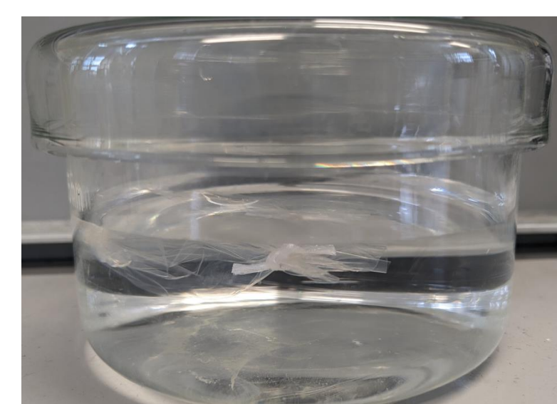
Figure 2. Dialysis bag containing PIL polymer mixture in deionised water.
